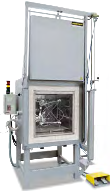
Holding frame for measurement of temperature uniformity
