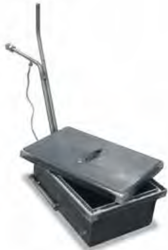
Annealing box with protective gas inlet and outlet
