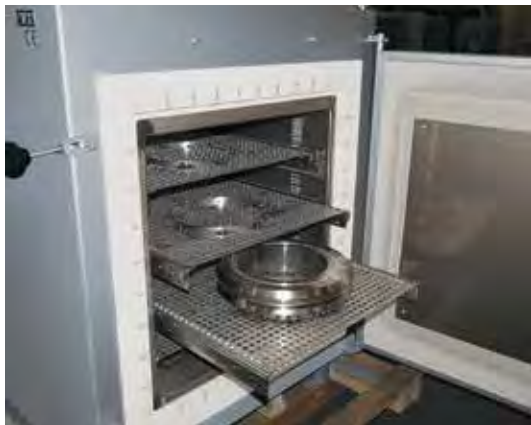
Forced convection furnace with charging grill shelves. The shelves can be moved individually on telescoping guides and can be taken out individually.
