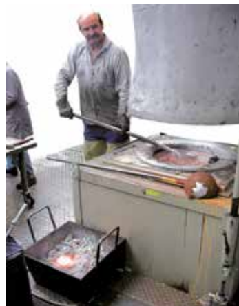
Manual ladling from a bale-out furnace T 80/10
